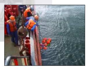
These moorings were recovered, serviced and redeployed in October from the vessel JV3 (pictured on left) and will be collecting data throughout the ice season. This metocean program is designed to provide engineering data for the design of ENG's offshore facilities.
