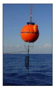
The oceanographic work scope involves the collection of currents at two deepwater stations and of currents and waves at two shallow water stations. Collection of current transect and CTD data is included at offshore visits. In addition, test pieces of the HDPE pipe have been moored to determine biofouling rates.
