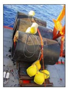
Each of the deep moorings (above right) is fitted with an RD Instruments 75kHz ADCP, Nortek Aquadopp current meter, RBR Ltd XR-420 CT logger and Argos satellite locator beacon. The shallow moorings are fitted with RD Instruments 600kHz ADCPs in bottom-mounted frames. Deployment and recovery of these frames is achieved with the use of Sonardyne lighweight acoustic release transponders.
