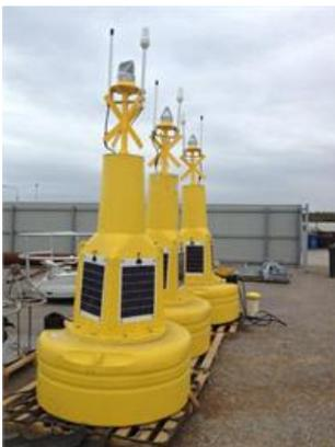
Metocean Services International (MSI) recently completed the installation of 3 real-time current profile monitoring buoys offshore Curtis Island at Gladstone in Queensland, Australia for Arrow Energy as part of a 3 year monitoring program.
