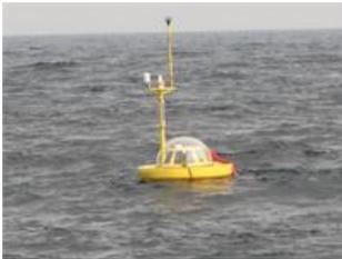
MSI is pleased to announce that it has successfully completed mobilisation of a current mooring, as well as a metocean buoy, for Maersk Oil Angola in Block 16 offshore Angola in approximately 1,200m water depth.
