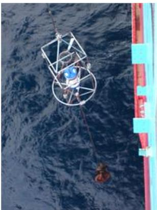
Metocean Services International (MSI) recently provided a real-time current measurement system for installation on the Maersk Guardian offshore Norway.
